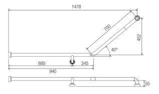
Drawn LH (Left Hand) Note: Horizontal flange connects directly to rear wall
